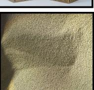
**ZEOLAN-K** is a mixture of 3A synthetic zeolites and natural binders. It is comparable with other zeolite based desiccants, however its low dust level and good flowability are important features.
